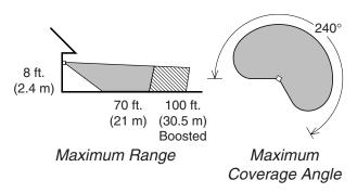
The detector is less sensitive to motion directly towards it.
